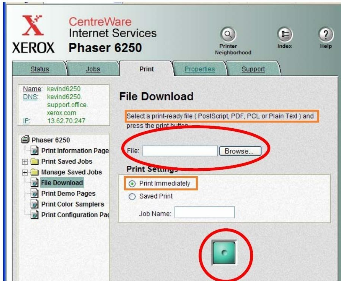
Figure 4: Select the firmware update file and press the green button to send it.
